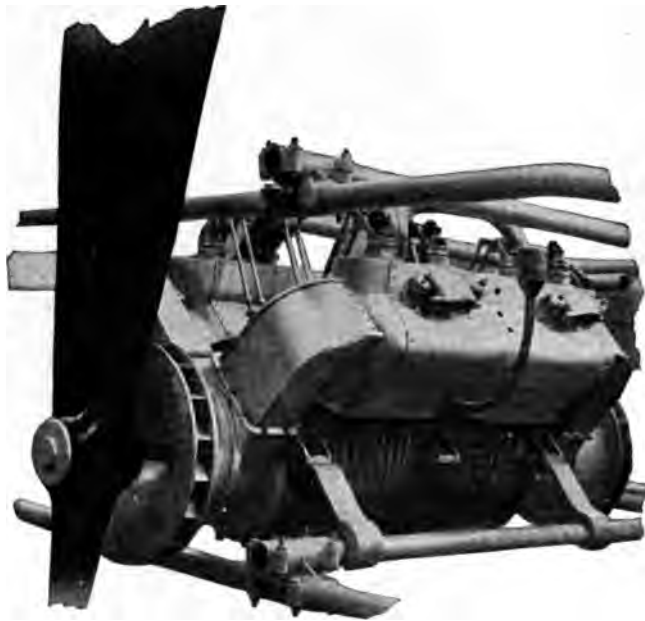
Fig. 36. Pipe Air-Jacketed V-Type Motor
